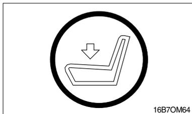
This LED lights when the operator is not on the seat.
