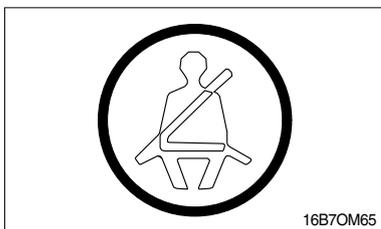
(1) This LED lights to signal that the seat belt is not correctly fastened. To connect the Seat belt sensor to the Analogue Input #2.
