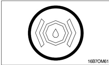
This LED lights when the measured oil level of the hydraulic circuit is under the minimum acceptable mark.
