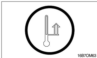
This LED blinks when one truck's controller is in alarm due IMS high temperature.
