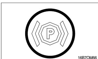
(1) This LED lights when the handbrake is activated.
